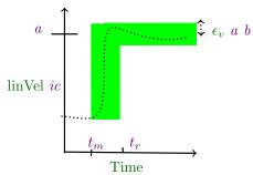
messages on the topic VELOCITY. It reacts to such messages by adjusting the speed of the two motors (one on each side) so the robot's linear and angular velocities are close to the requested values. The figure above illustrates how the linear velocity of an iCreate is supposed to change in response to a message requesting a linear velocity a and angular velocity b.  $t_m$  denotes the time when the
